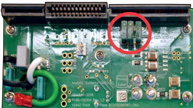
Pictured: Front panel circuit board. Output fuse location indicated by red circle.
