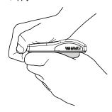
Apply 12V DC label, and circuit labels. Remove fuse seal and check that appropriately rated fuses are installed for each device.
