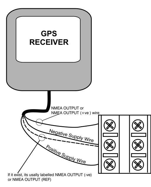
If not, then the reference is internally connected to ground, and can be ingnored
