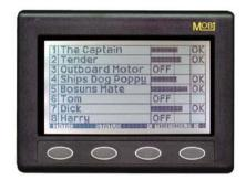
In operation the base station sequentially interrogates each transponder which then broadcasts its presence. In the event of a crew member falling overboard the drop in signal level is detected by the base unit which sounds a high intensity audible alarm.
