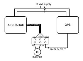
Connect the NMEA output (or NMEA +) of the GPS to the BLUE wire of the UTILITY cable. If the GPS has a NMEA - or NMEA REF connect this wire to the vessel supply negative. The AIS radar requires an NMEA 0183 signal with RMC sentence. The signal level must swing above and below 2 volts.
