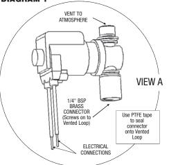
NOTE: The switch on the side of the solenoid is inactive and will not affect operation.
