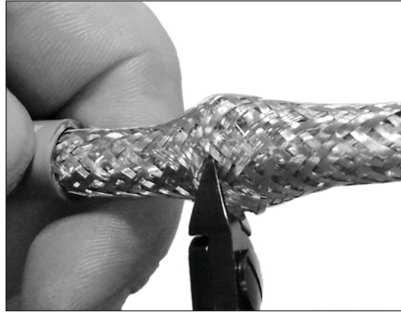
Figure 34 Cable Braid Bulge/Cutting
