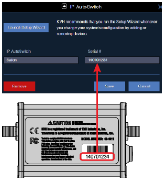
Figure 7-2 Adding an IP AutoSwitch to the Autoswitch Page
