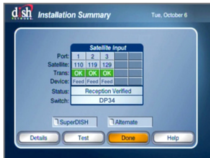
Figure 5-8 Check Switch Test Results
