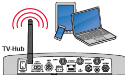
Figure 2-5 Wireless Connection to TV-Hub Web Interface
