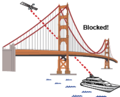
Figure 2-2 Example of Satellite Blockage
