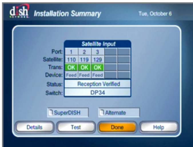
Figure 5-7 Check Switch Test Results
