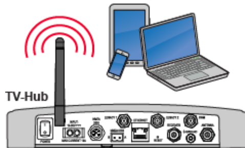
Figure 3-3 TV-Hub Wi-Fi Connection (TV-Hub A shown)
