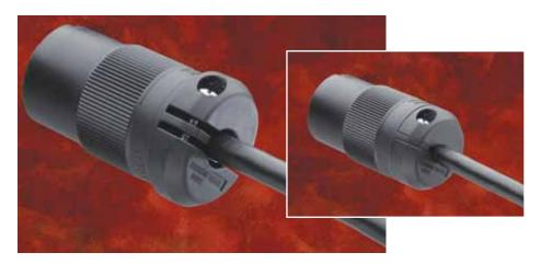
Clamp-Lock devices feature a self-centering cord grip for faster assembly. A molded-in guide shows how much wire should be stripped.
