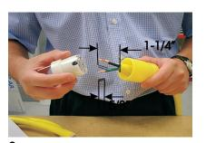
2 Slide housing over cord. Strip 5/8 in. of insulation off each of the three wires. Make sure the wire is clean and a bright copper color. Do not solder the ends of the wire.
