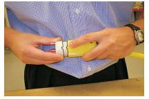
**4** Recouple the two sections by aligning the key with the key slot.
