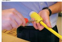
**6** Tighten cord clamp by tighten two assembly screws to 16-20 inch-pounds torque.
