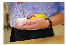
**3** Insert bare wires into their corresponding color-coded terminals. Make certain there is not wire insulation under any terminal clamp. Tighten the screw clamps to 14-20 inch-pounds torque.
