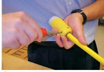
**6** Tighten cord clamp by tighten two assembly screws to 16-20 inch-pounds torque.
