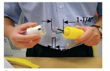
2 Slide housing over cord. Strip 5/8 in. of insulation off each of the three wires. Make sure the wire is clean and a bright copper color. Do not solder the ends of the wire.
