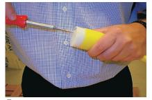
**5** Tighten down the recessed screws with moderate torque.
