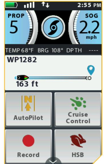
The Go To Waypoint Active Band appears when the boat is navigating to a saved Waypoint. The Waypoint 1282 is 163 feet away.
