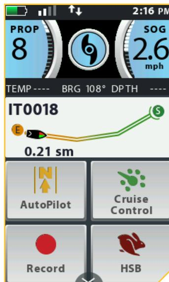
The iTrack Active Band appears when a Go To iTrack action is taking place. The current To Start location on the iTrack being navigated is 0.21 statute miles away.
