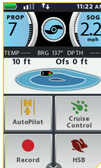
The Follow the Contour Active Band appears when the boat is navigating with Follow the Contour. The Contour being followed is 10 feet. The Offset is set to 0 feet.
