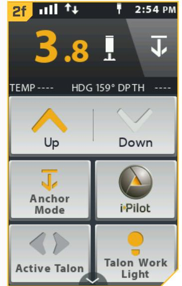
**NOTICE:** Unless the Talon Control setting on the i-Pilot Link Remote is set to Right or Left, the remote will control both Talons when deploying. Be mindful of which Talon(s) is selected when deploying them.
