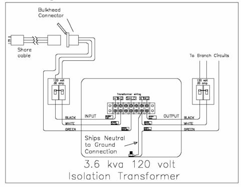
30 amp/120volt/60hz U.S. Polarization Transformer Wiring Diagram using 3.6 kva Transformer
