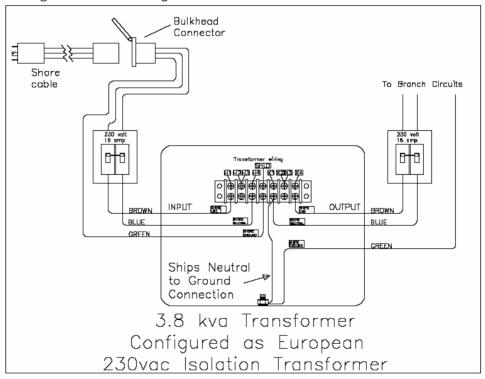
16amp/230volt/50hz European Polarization Transformer Wiring Diagram using 3.8 kva Transformer
