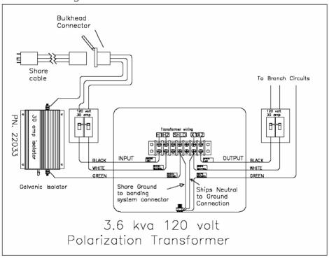
30 amp/120volt/60hz U.S. Isolation Transformer Wiring Diagram using 3.8 kva Transformer
