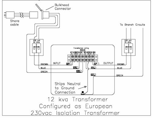
32amp/230volt/50hz European Polarization Transformer Wiring Diagram using 12.0kva 50/60hz Transformer
