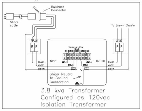
30 amp/120volt/50hz U.S. Polarization Transformer Wiring Diagram using 3.8 kva Transformer
