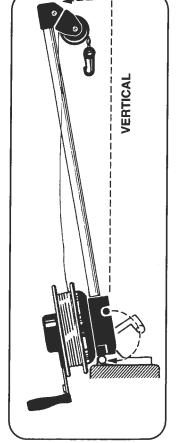
Red lock lever must be tucked under base to lock the downrigger upright
