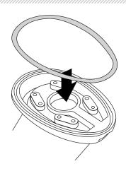
Place the ADA-FN-M1 ontop of the mount, be sure to line up the four mounting holes.
