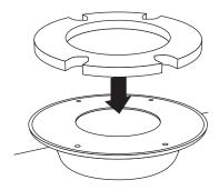
Mount the satellite dome ontop of the foam gasket.
