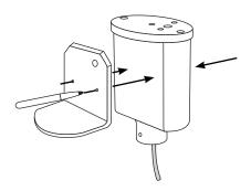
Using a drill bit drill the holes you just previously marked on both sides.
