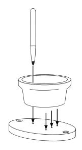
Using a drill bit, drill the holes you just marked.
