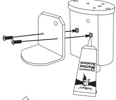
Using marine adhesive sealant apply some around the two holes and perimeter of the top as shown.
