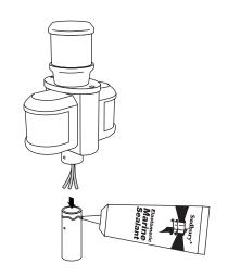
Apply marine adhesive sealant around the front and back holes as shown.
