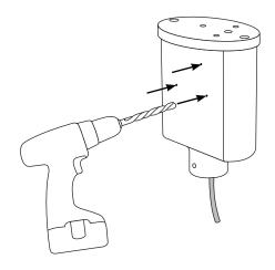
Using the hardware that came with your light, secure lights to the front and back of the LTB-BOX or LTB-BOXW.
