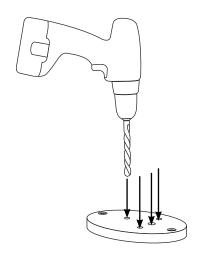
Place the lighting bracket on the face of the LTB-BOX or LTB-BOXW. Then mark the necessary holes for drilling. Repeat on other face.
