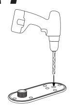
Apply marine adhesive sealant around the holes that you drilled for the light assembly. Secure the light assembly. You may be able to use one of the provided screws.
