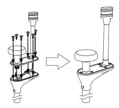
Apply marine adhesive sealant around the top of the Light bar as shown, then slide the LTB-U1A on to the Light Bar.
