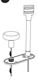
Apply marine adhesive sealant around the top of the Light bar as shown, then slide the LTB-U1A on to the Light Bar.
