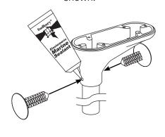
Apply marine adhesive sealant into the groove of the LTB-U1A as shown.
