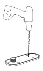
Mark the enter cable hole for drilling.
