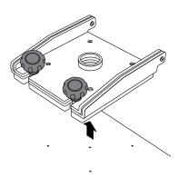
Drill the four bolt holes using a 5/16" drill bit.
