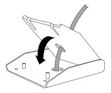
Fold the knobs back over and tighten to secure the two plates of the biggs. of the hinge adapter.
