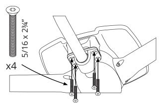
NOTE: Use 4 each of the 5/16" x 3" bolts when installing a light bar if your top plate is 3/4" or thicker.
