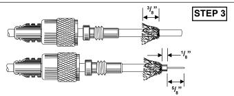
Fan the braid back, as illustrated, and trim it to 3/8". Strip the insulation from the center conductor as shown. **Be careful not to damage the center conductor.**
